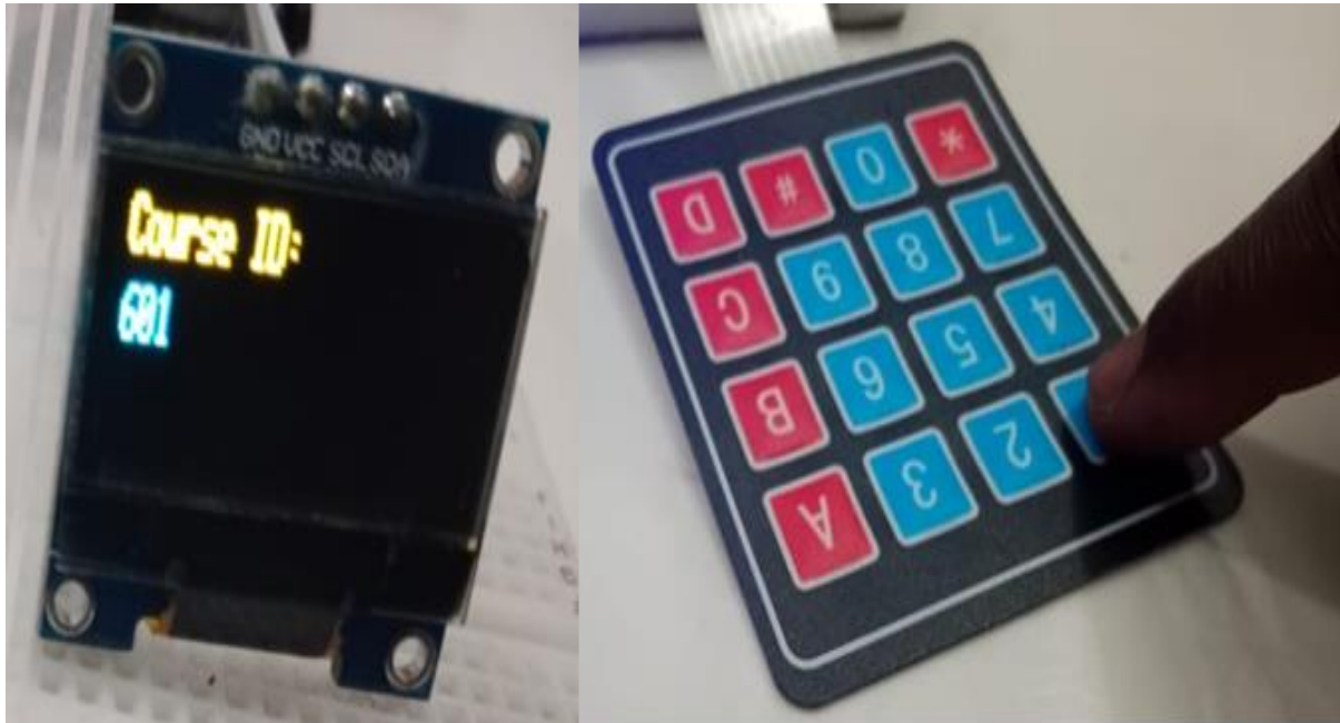
Figure 6 The picture showing the keying in of the course ID using the keypad
